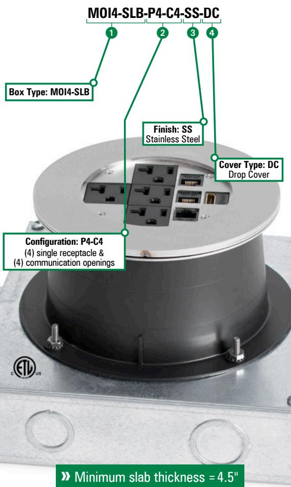
» Minimum slab thickness = 4.5"
